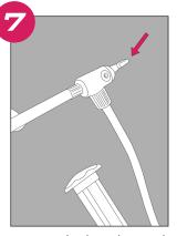
Connect both ends together and then lock the air pump if applicable.
