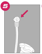
Connect this air-pump nozzle to one of the ends of the air pump extender.
