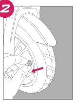
Remove the air cap turning it counter-clockwise
