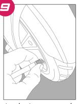
Attach air-pump extender to the tire nozzle and rotate it clockwise to lock it. Begin pumping air.
